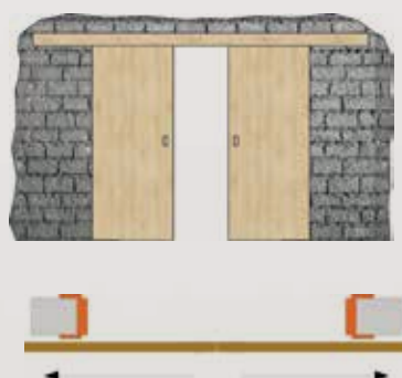
DOUBLE-LEAF DOOR OPENING PARALLEL TO THE WALL
